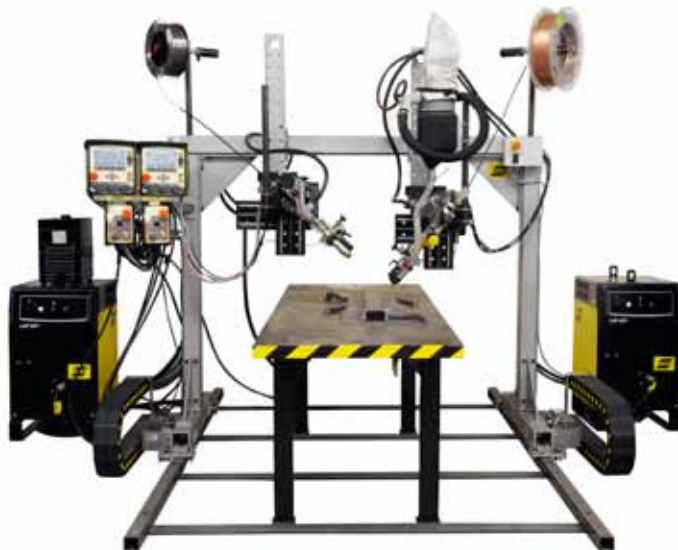
Mechtrac equipped with A2 welding heads, process controller PEK and power sources LAF 631
